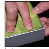
Repeat Step 1 for opposite corner C, then insert corner B, followed by corner D. to complete the installation of the corners
