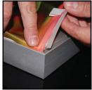
Insert corner A. Turn edge of graphic so silicon welt is perpendicular to face of graphic. Insert narrow side of welt with fabric to outside into the channel. Repeat for other side of this corner.
